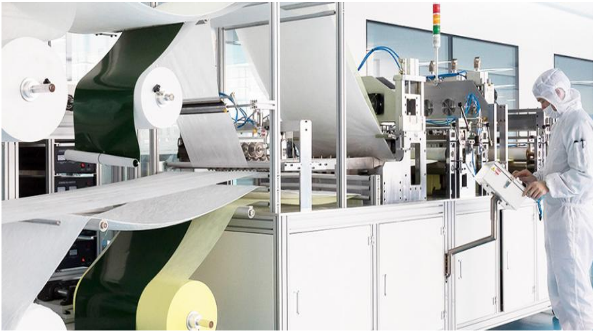
Welding production line for pre-filer
