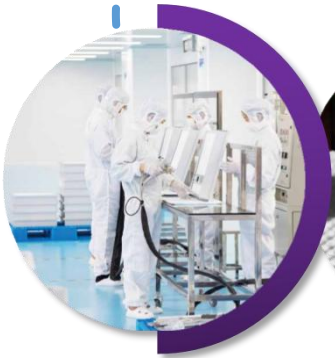
10 HEPA filter gluing process
