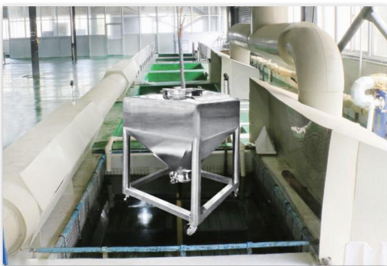
Degreasing, washing, surface conditioning, phosphating
