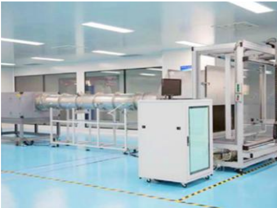
MPPS test machine According to EN1822
