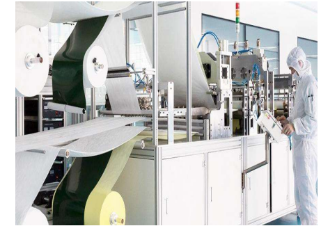
Pre-filter production line
